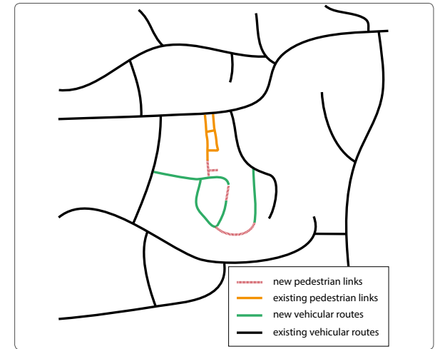
Fig 3.3.13 - Early 2000s – modern infill with good connectivity and linkages to surrounding streets and spaces.
