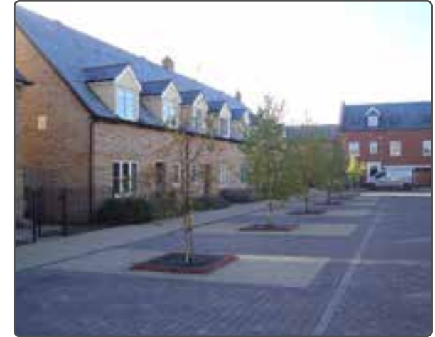
The use of street trees helps to define car parking spaces - Cambourne
